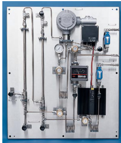
Moisture analysis in high pressure natural gas. Dual coalescing filters with bypass flow to remove TEG from sample gas. (TEG is conductive alcohol found in pipeline NG from TEG dryer carryover, which can bias Alux sensor readings.) It can be coalesced out of sample, providing reliable sensor performance
