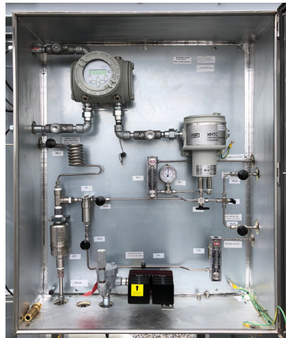
Thermal conductivity binary gas analysis with hazardous area display and heater for outdoor biogas analysis.
