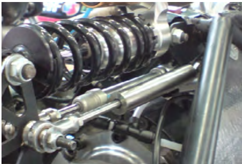
APPLICATION: S-SERIES TRANSDUCER MONITORING AUTO FRAME
