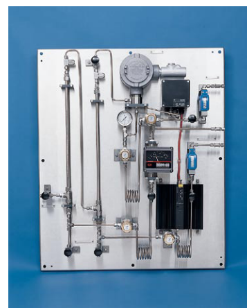
Moisture analysis in high pressure natural gas. Dual coalescing filters with bypass flow to remove TEG from sample gas. (TEG is conductive alcohol found in pipeline NG from TEG dryer carryover, which can bias Alux sensor readings.) It can be coalesced out of sample, providing reliable sensor performance.
