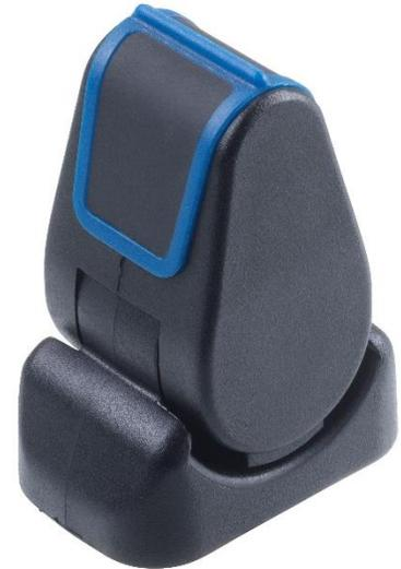
The JC1210 builds on the success of the JC1200 and incorporates the same robust design with exceptional life and now offers the option of overpress and latch features at the ends of travel. This new joystick utilizes non-contacting, Hall-effect sensing technology for long-life integrity of the output signal. Operating feel has been an important part of this new development to make this unit as smooth and easy to operate as possible throughout a 5 million cycle life to the start of overpress
